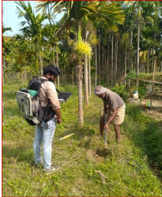
Measurement of Soil Spectra using Spectro radiometer at Palakkad
