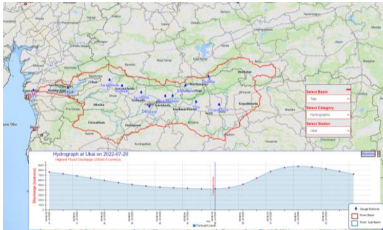
Computed flood hydrograph at Ukai Dam, Tapi River (21 Jul 2022)
