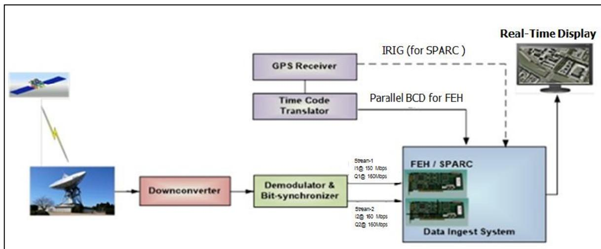
**Figure-27 FEH in Ground Receive chain**
