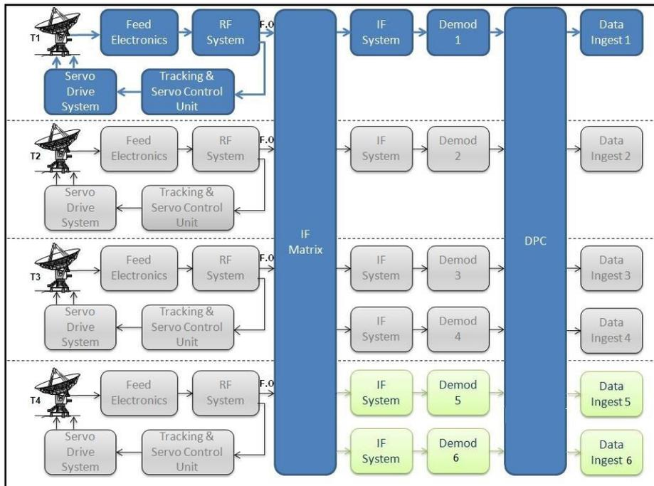
**Figure-19 IMGEOS Configuration of Data Reception Station**
