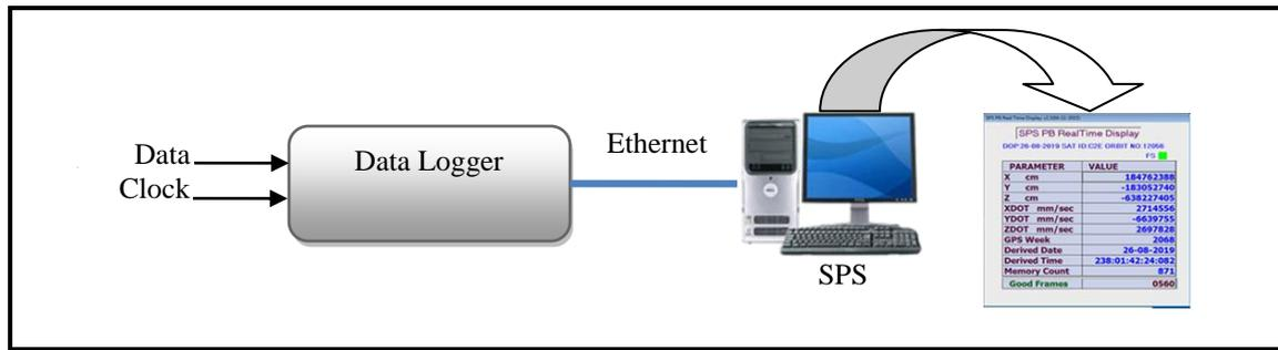
Figure-23 SPS Data Archival System based on TCP/IP
