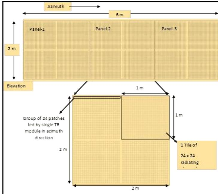
**Figure-8 Distributed antenna for high resolution SAR**
