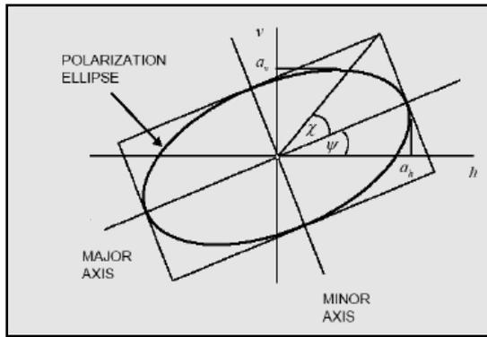
**Figure-4 Polarization Ellipse**
