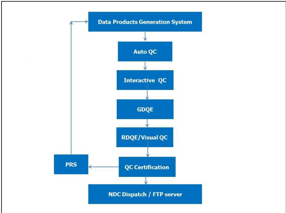
**Figure-34 Data products verification and certification**
