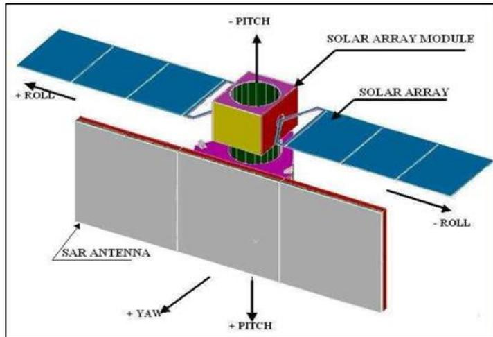
**Figure-10 Deployed Configuration of EOS-04**
