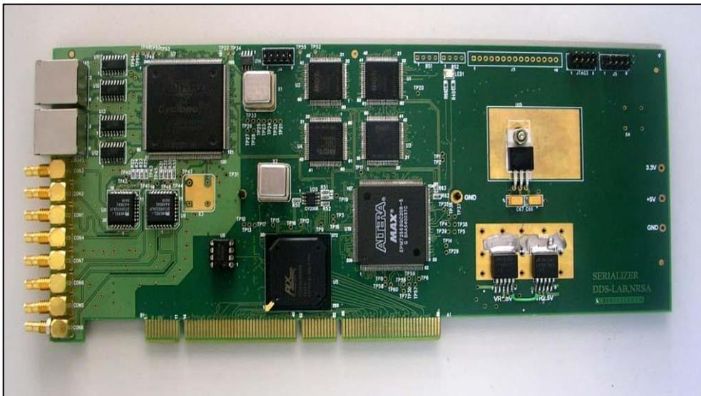
**Figure-29 PCI Serializer card**
