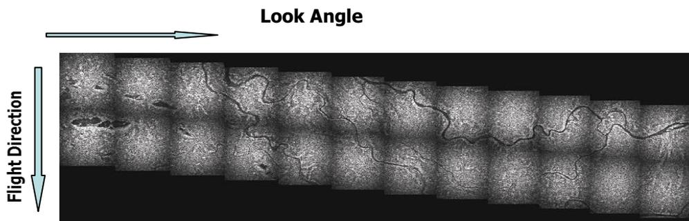
**Figure-13 Illustration of Scalping in a Simulated Image**
