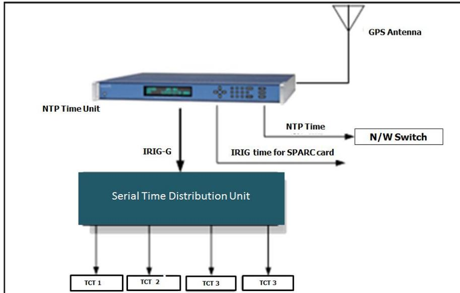
**Figure-25 Timing System Block Diagram**
