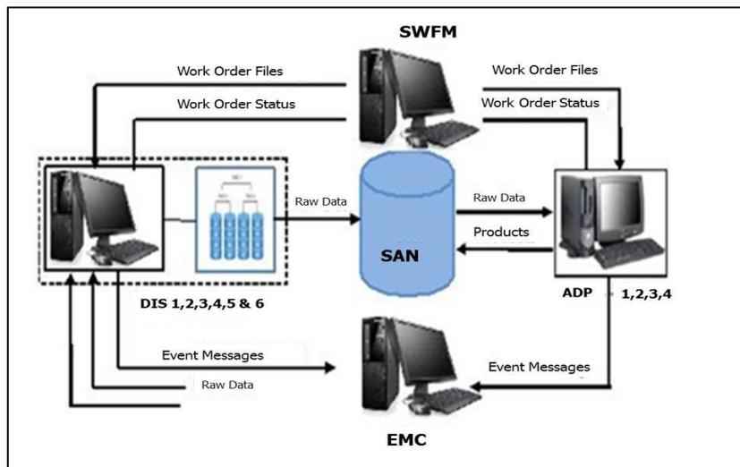
**Figure-21 Block Diagram of Level-0 Systems Configuration**
