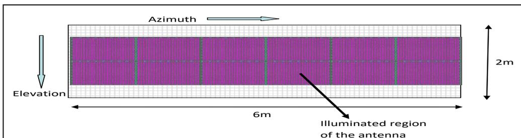
**Figure-9 Change of antenna electrical width to cater to variable elevation**
