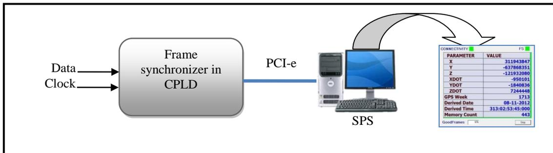
Figure-24 SPS Data Archival System based on Adlink PCI-e
