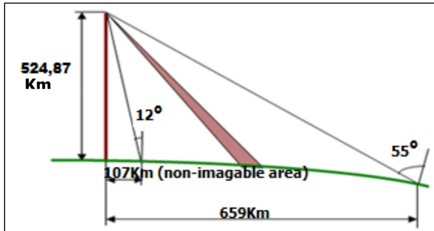
Figure-6 Basic system geometry
