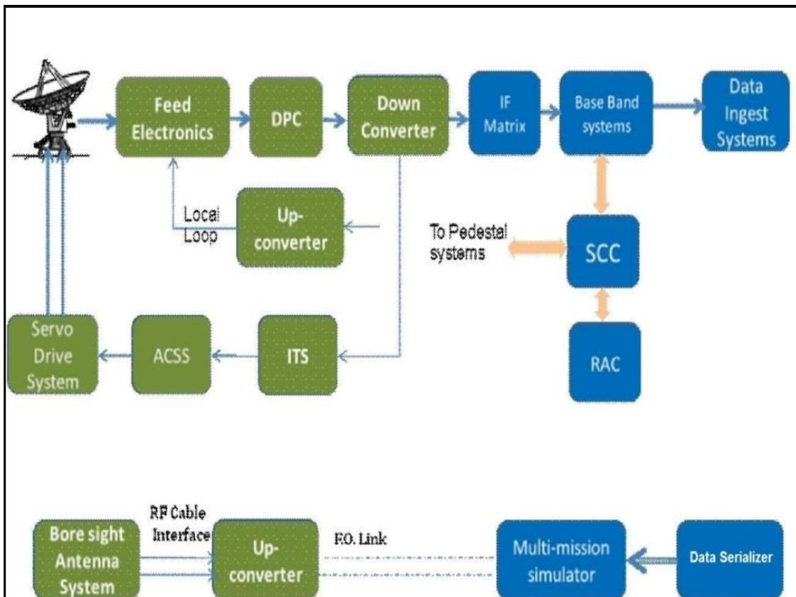
**Figure-20 Configuration of Data Reception Systems**
