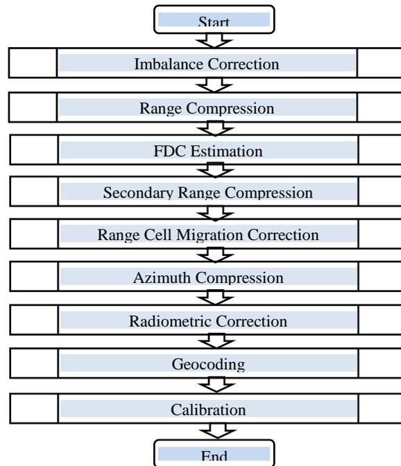
Range compression, RCM correction and azimuth compression are core image formation steps in SAR.
