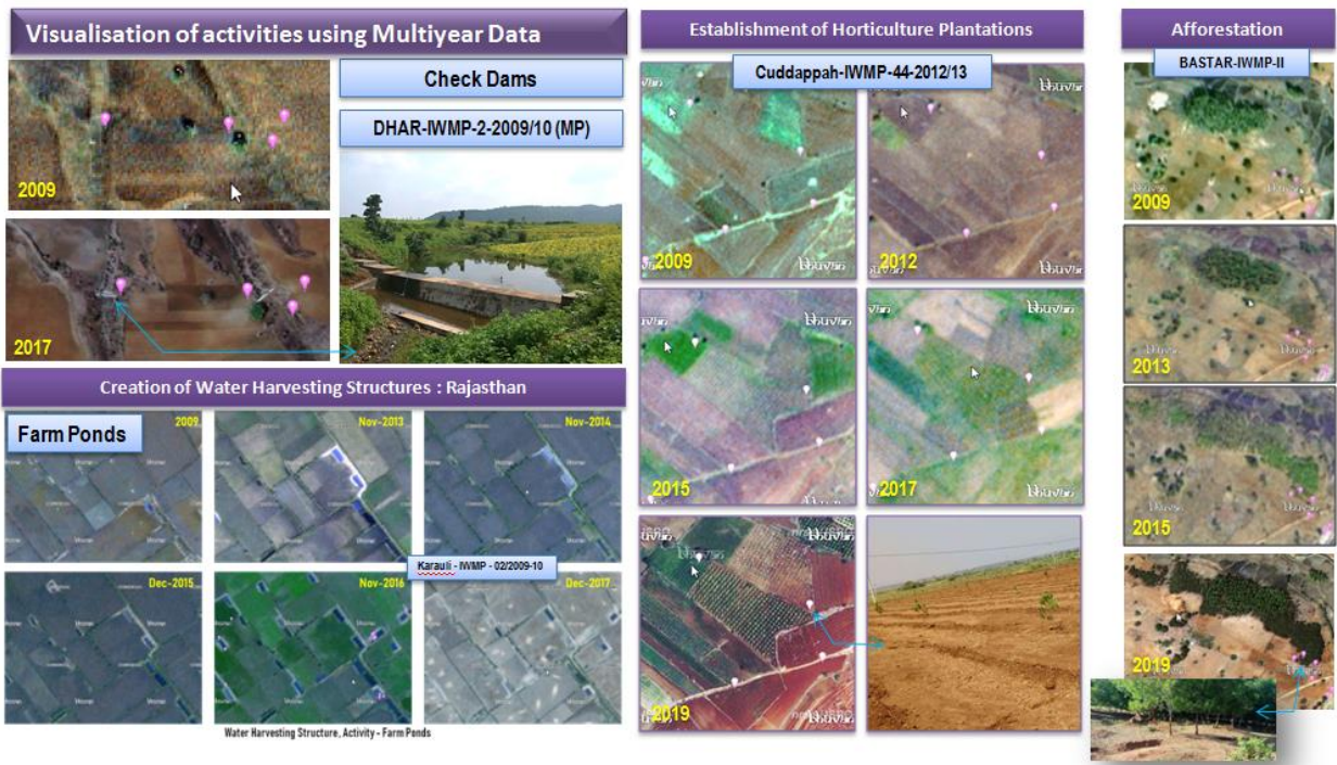
The impact of interventions by Watershed development activities as observed using a high-resolution multi-temporal image sequence. Check dams, Water Harvesting Structures, Horticulture Plantations, and forestry species are analyzed.
