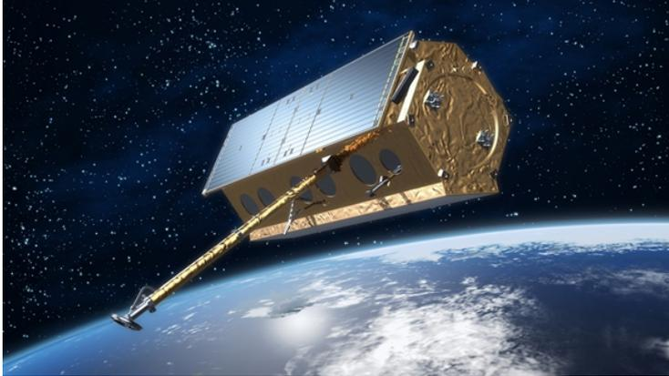
The German radar satellite TerraSAR-X will orbit the Earth in a polar orbit at a height of 514 kilometres; using the mission's newly designed active antenna, it will gather high-quality X-band radar data from the entire planet. TerraSAR-X will operate independent of weather conditions, cloud coverage or lighting and will supply radar data at a resolution of up to 1 metre.
