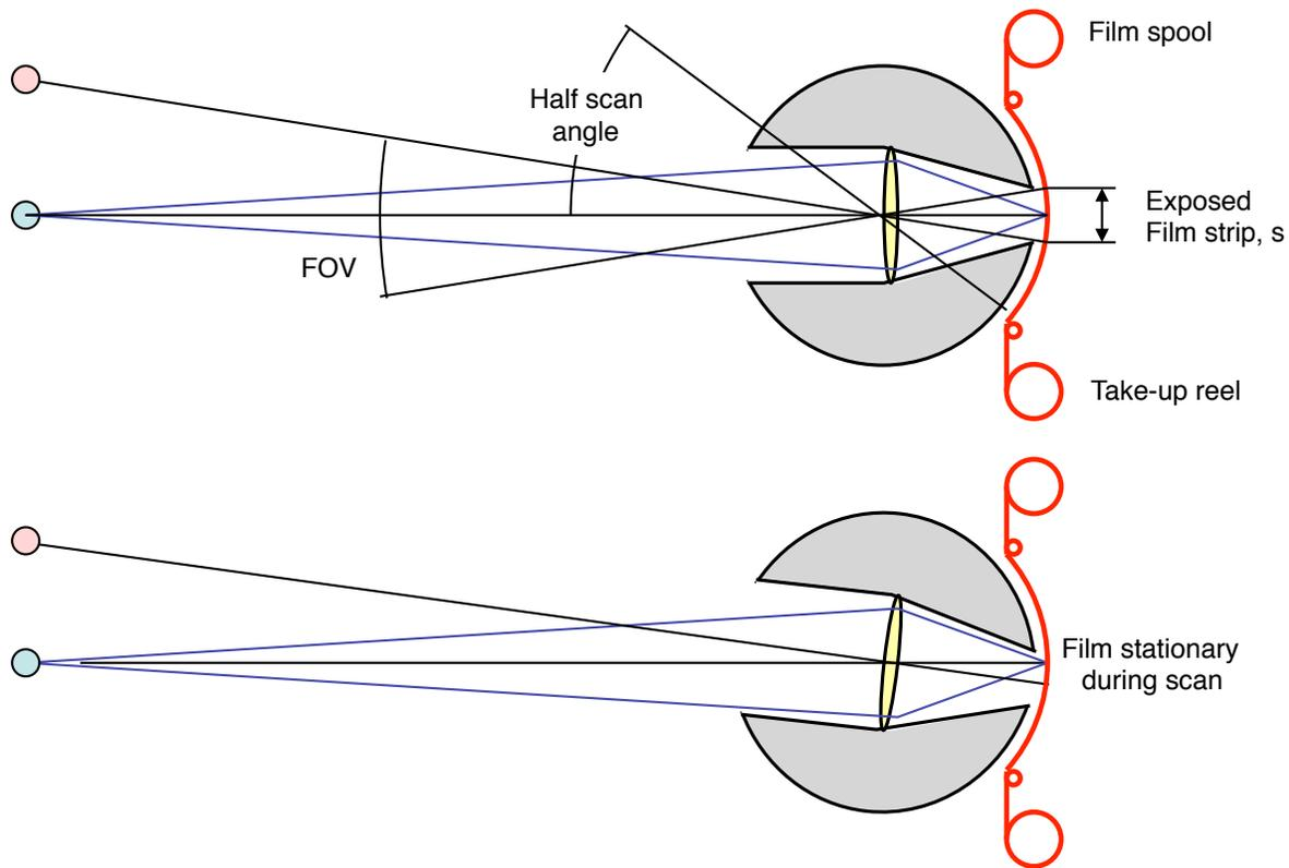
Figure 5. Swing Lens Panoramic Camera Concept.
