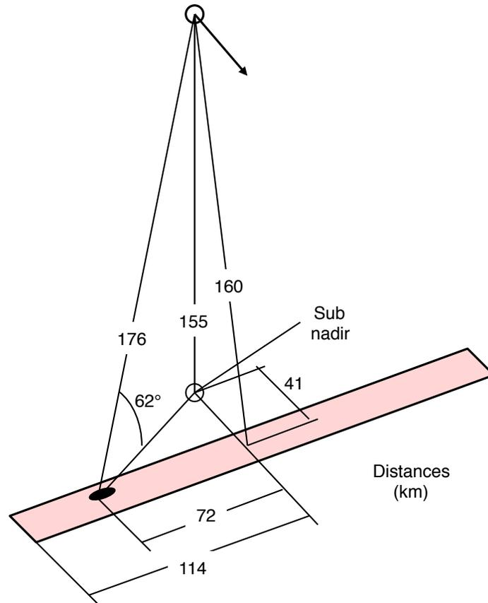
Figure 10. Viewing Geometry for Frame 28. The left of center dot in the scene locates Washington DC some 72 km from the center of the frame.
