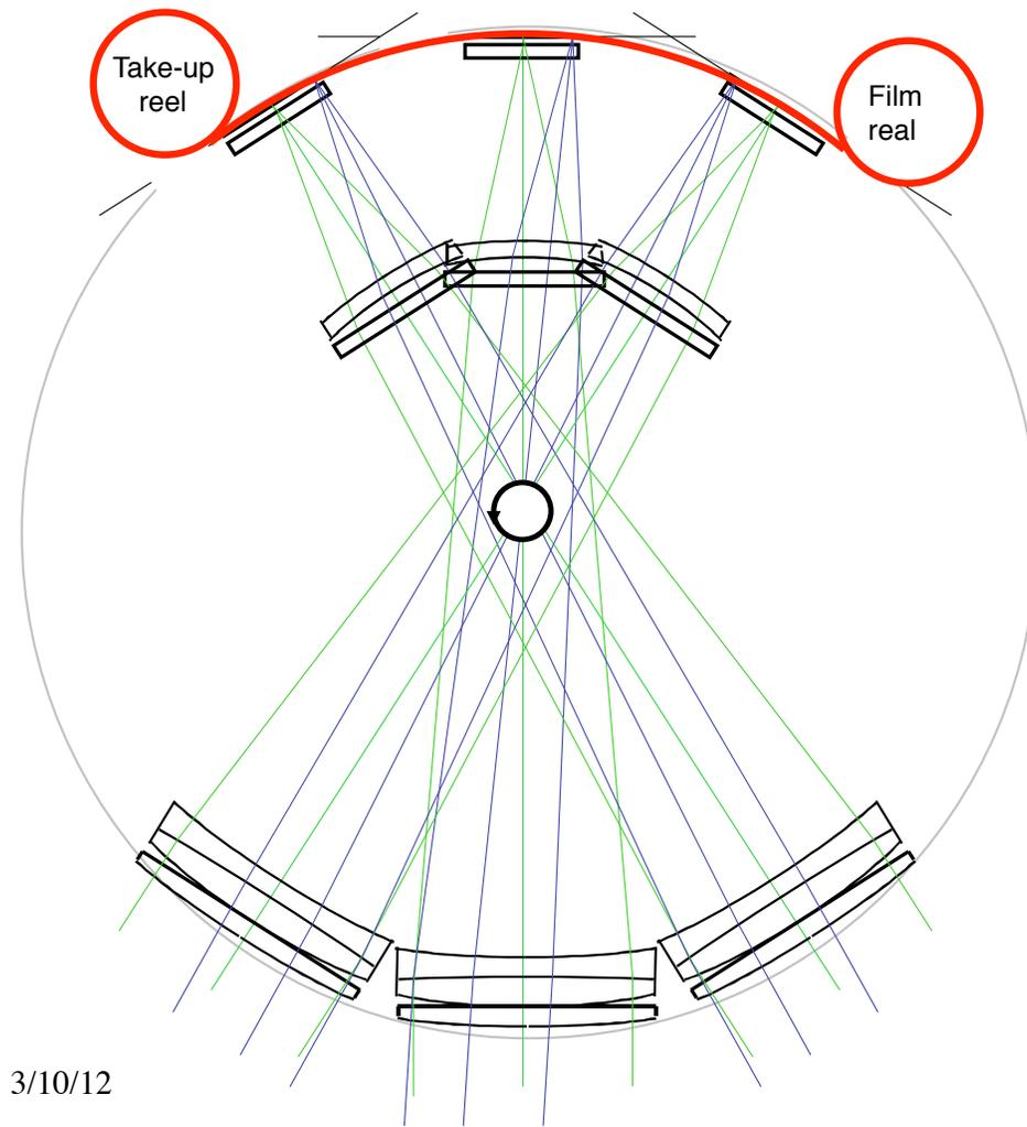
Figure 7. Rotation About the Nodal Point for a Petzval Lens
