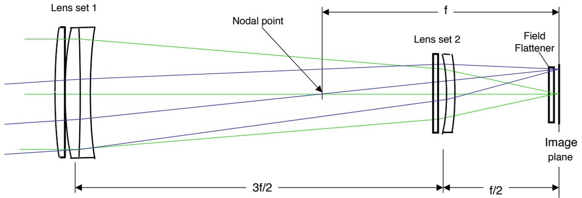
Figure 6. Petzval Lens (Approximate Representation of Corona Design)
