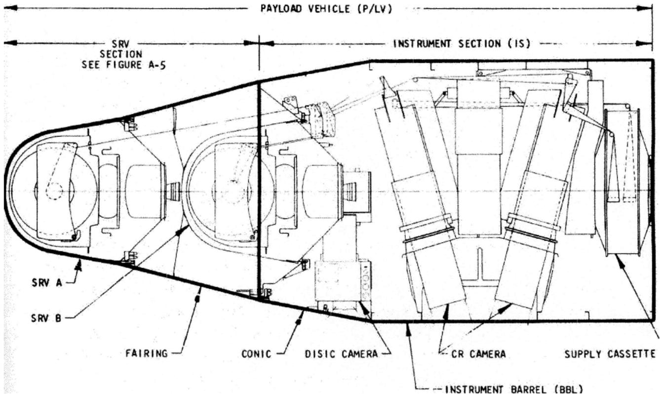
Figure 3. Schematic of Corona KH-4B Payload (national air and space museum, nasm)
