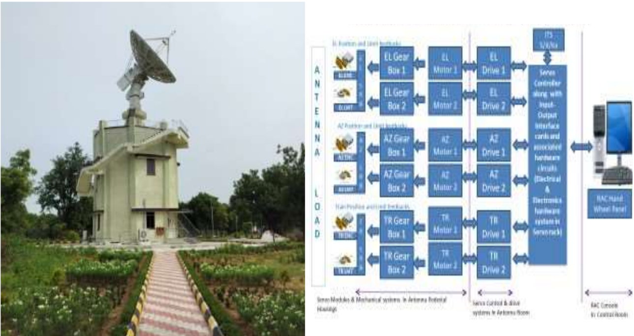
Fig.1 Block diagram of the ACSS along with tri-axis antenna
